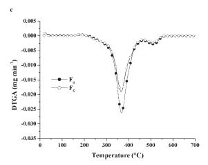
Figure 2. DTGA in air, 10  $^{\circ}$ C min $^{-1}$ : (a)  $A_o$ ,  $A_s$  (b)  $E_o$ ,  $E_s$  (c)  $F_o$ ,  $F_s$ .
