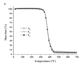
Figure 1. In N<sub>2</sub>, 10  $^{\circ}$ C min<sup>-1</sup>: (a) DTGA A<sub>0</sub>, A<sub>5</sub>, (b) TGA A<sub>5</sub>, E<sub>5</sub>, F<sub>5</sub>.
